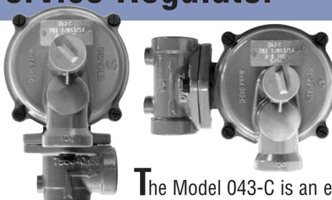
The Model 043-C is an excellent general purpose gas pressure regulator. It can be used for natural gas, air, CO<sub>2</sub>, propane, butane, nitrogen, and other gases. It can be used for gas services to homes, commercial establishments and small industries, for burners, unit heaters, boilers, and other equipment. The Model 043-C includes an internal relief valve.
